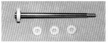
☐ FIG. 113—In a separate bag will be six nylon spacers. Slip three of these onto each of the long shafts, all the way up to the piston. These spacers are not used on the front shocks.
