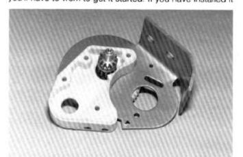
fingers and try to turn the big plastic gear. It should be VERY HARD to turn.
